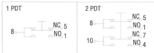
Form "C" Switch Circuits
