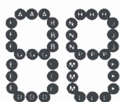
TYPE D FRONT VIEW 4-Segment and TWO 7-Segment Designations
