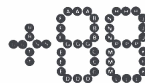
TYPE G FRONT VIEW THREE 7-Segment Designations
