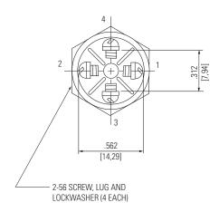
Mounting and terminal hardware supplied unassembled.
