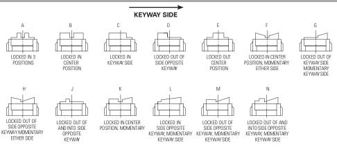
Figures A thru N do not represent details of construction. They schematically illustrate locking function
