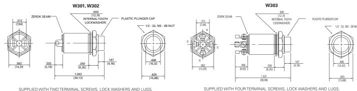
SUPPLIED WITH TWO TERMINAL SCREWS, LOCK WASHERS AND LUGS.
