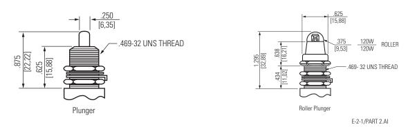
Plunger Operated - As with all push-on units, this actuator has an ice scraper for clearing the plunger of ice and debris with each operation.
