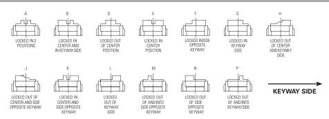
Figures A thru P do not represent details of construction. They schematically illustrate locking function.
