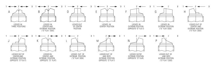
Notes: 1. Arrows (<>>) indicated lever must be unlocked to move against the arrow direction.
