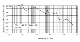
Graphic Illustration defines relative shielding efficiency of RFI shielded component/ components over unshielded device.
