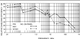
Graphic Illustration defines relative shielding efficiency of RFI shielded component/ components over unshielded device.
