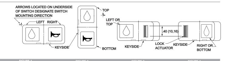
Horizontal Mount Vertical Mount Locking Actuator Styles 4, 5, Y, & T Locking Actuator Styles 6, 7, W, & S
