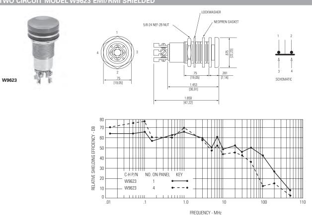
Graphic illustration defines relative shielding efficiency of RFI shielded component/ components over unshielded device.
